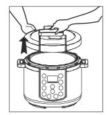
To mount the lid, place it at a distance of 10cm above the body of the appliance, tilt it toward the socket [housing] and turn clockwise. The lid is mounted.
