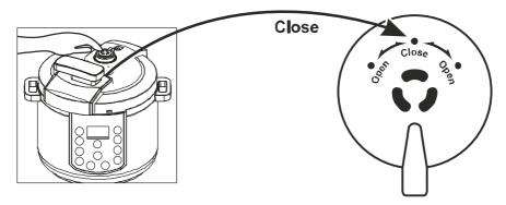
**Note:** To cook in multicooker mode, the pressure valve is not required to be place in the "Closed" position.
