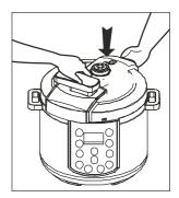
**CAUTION:** Before you close the lid, make sure the silicone gasket is not missing from the lid. Do not use the appliance without this gasket.
