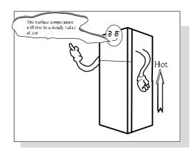
30 minutes later, open the freezer compartment door, feel the cold air, that means the unit works properly.
